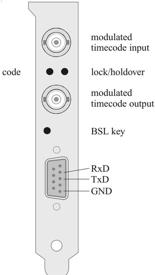
The bracket of the board includes the BNC-connectors for the amplitude modulated time codes (input/output), two LEDs, a key for activating the Bootstrap-Loader and a 9 pin D-Sub-plug.
